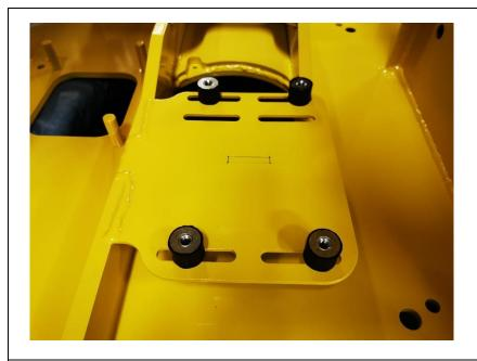
Place the 4 silentblocs with a Ø8x30 washers and a M8 locknut for each; do not tighten them now as it will be easier to install the engine this way.
