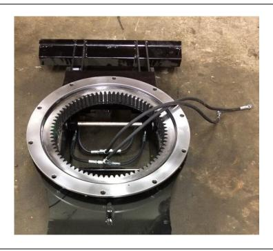
Place the slewing ring on the frame and bolt it down with 16 M12x30 bolts
