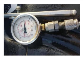
Tighten every connection by hand then start the engine.
