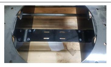
Install the rotary joint support plate at the center of the frame.
