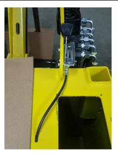
Lubricate the cable with a little oil on each end of the sheath.
