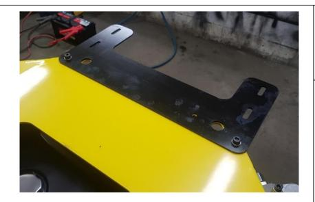
Install the radiator support plate.
