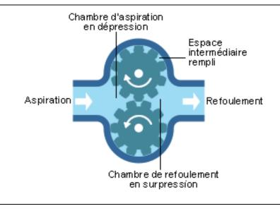
Before locking the lantern in position, check the direction of rotation of the pump, for this, take off the plugs and slowly pull on the motor's starter rope. Look from on side in the pump:
