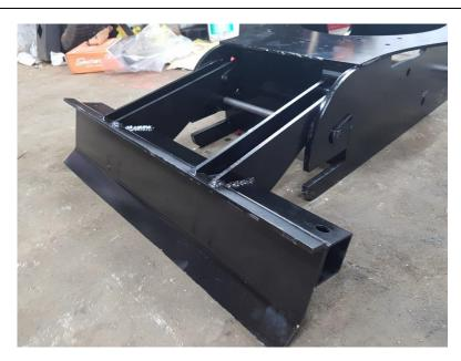
Install the blade with an Ø25 mm lengh 435 mm teardrop pin from one side to the other of the base frame.
