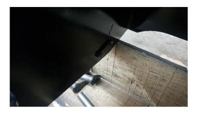
Lock the teardrops at on the other side with 2 M6x16 botls and threadlocker.
