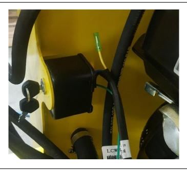
Take the contactor off the motor, cut off the 2 brackets and screw it through the front of the turret.
