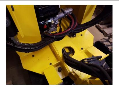
Once the system is tested, assemble all the hoses with cable tie.
