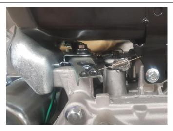
Loosen the nut on the accelerator until the lever can move without restrictions.
