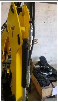
2 fittings AT12L-12x17 to screw on the cylinder's elbows then 2 UM12L-15x21 on the hoses.
