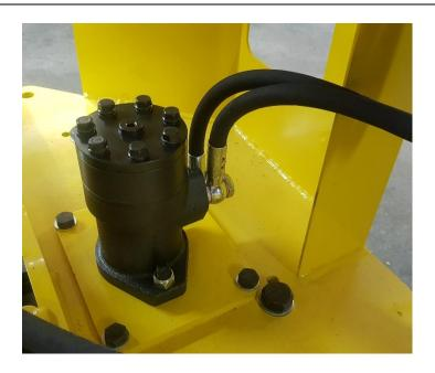
Place the reduction with teflon then connect the hoses to the distributor.
