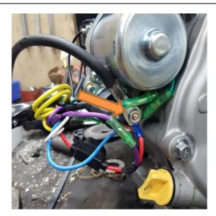
Connect the + to the back of the coil where the red cable is already connected.
