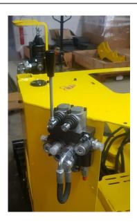
Place the 2 elements distributors at the back of the turret. One joystick spring back in position, put a bypass on this one, the other one stays in place, connect this one according to the guide p 40.
