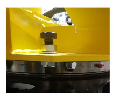
Turn back the turret to its original position and install the stop bolt; it can be placed on either side of the swing bracket.
