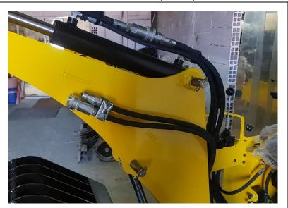
The hydraulic lines for the telescopic arm are 2 hoses connected from the distributor instead of the bypass 15-16 going to the telescopic arm.
