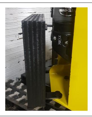
Place the first plate on the pivot axis with a  $\emptyset$ 20 lg 430 teardrop shaft and lock it with a 6x16 bolt on the turret.
