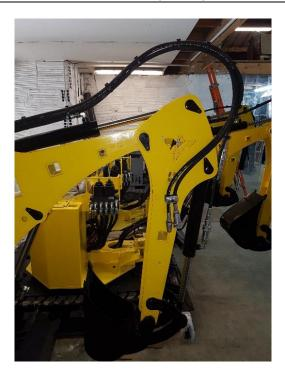
The hydraulic line to the tip of the arm are 2 hoses connected from the distributor instead of the bypass 15-16 going to the telescopic arm.
