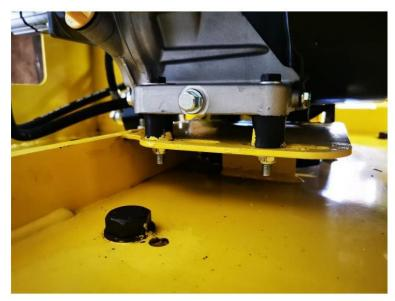
Place the engine on the silenbloc and fix it with 4 bolts M8x35 and washers. Once the 4 bolts are in place, tighten everything.
