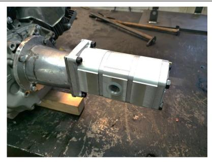
Place the pump on the lantern with 4 BTR 8x30 bolts and threadlocker.
