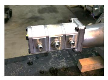
Place 2 fitting UM12L-12x17 on the sides and 1 fitting UM12L-15x21 in the middle.
