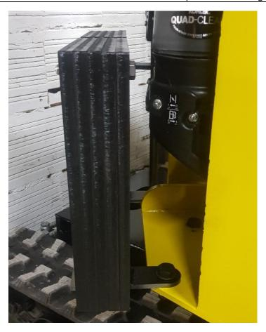
Place the first plate on the pivot axis with a  $\emptyset$ 20 lg 430 teardrop shaft and lock it with a 6x16 bolt on the turret.
