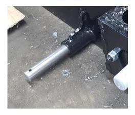
To ease the installation of the rollers, one can sand the shafts and coat them with grease.
