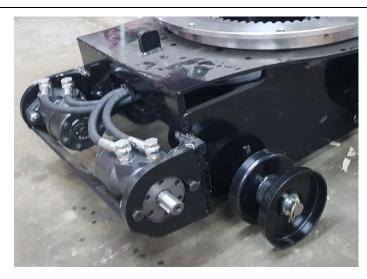
Before installing the rubber track, place the gear on the hydraulic motor and adjust if if need be.
