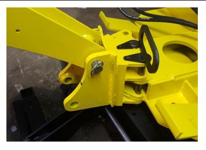
Place the slewing bracket with a  $\emptyset$ 25 lg 210 shaft in the center and a  $\emptyset$ 25 lg 210 shaft with a handle on one of the sides.
