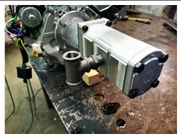
Place the low pressure ¾ T on the pump with Teflon.
