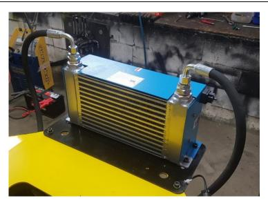
Connect the hoses from the distributor to the radiator then to the tank. See Diagram page 36-37.
