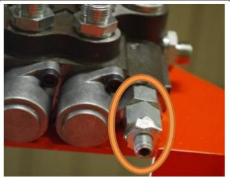
If the excavator lacks power or is under the recommended pressure, you need to adjust the pressure by fist taking off the metal cap on the pressure relive valve then with an allen key screw ¼ turn at a time to raise the pressure or unscrew ¼ at a time to lower the pressure. Do not overtighten as it may cause problems on the hydraulic system.
