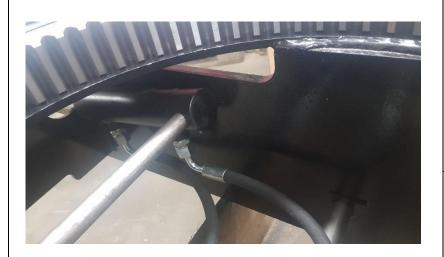
Place the 25x40 c 100 cylinders in the frame with the fittings UM12L pointed downwards and fix the back of the cylinders with a teardrop shaft Ø20 lg 435.
