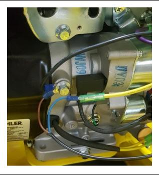
Connect the cable to the Kohler motor, the black cable to the mass and the red cable to one of the motor's yellow cable (+12 V after ignition).
