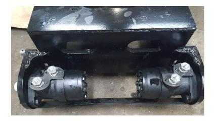
Put with teflon 2 reductions MC1/2-F3/8 on each motor.
