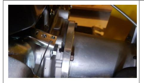
Pass the cable in one of the holes of the accelerator and bend it in place.
