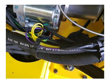
Plug the + terminal of the hourmeter to one of the available yellow wire of the Kohler motor (the 2 yellow wires are + at 12 Volt).
