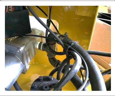
Connect the 2 supply hoses from the tank to the pump.
