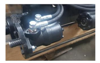
Connect the hoses to the hydraulic motors.
