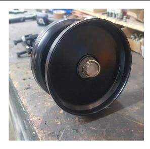
Add 1 pin on each side so that the roller does not slide off the axle.
