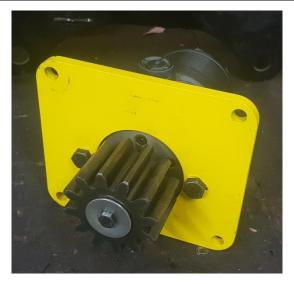
Add the gear to the motor's shaft and lock it in place with a 8x40 bolt + washer and threadlocker.
