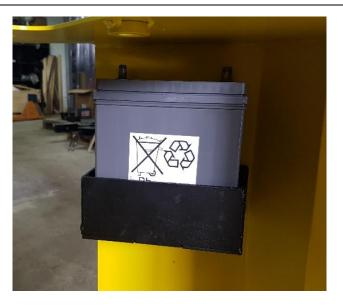
Before installing the engine in the turret, place the battery and support with 2 M8x20 bolts and locknuts.
