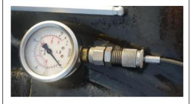
Place the female union ¼ on the manometer and screw the flexible capillary on it.
