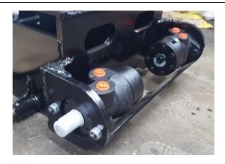
Install 2 hydraulic motors OMR200 on the frame with 2 M12x50 bolts with 2 brake nuts for each motor.
