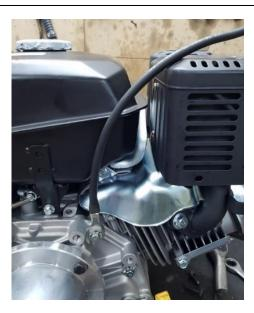
Connect the 25 cm cable to the mass at one of the motor's casing bolts.
