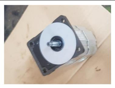
Place the centering washer on the pump.
