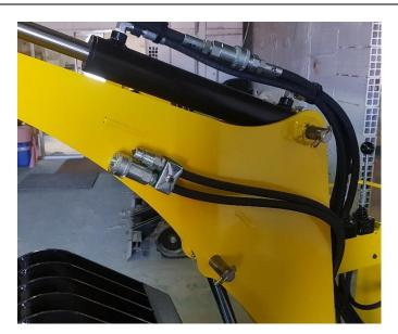
Install the auxiliary hydraulic line from the rear distributor and fix it on the side of the boom.
