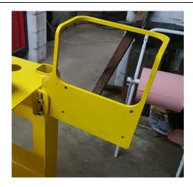
Install the distributor's support on the turret, the height can be adjusted later.
