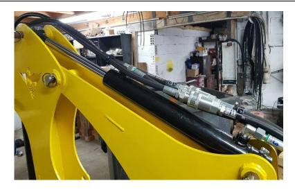
Install tightly the quick coupler on the hoses 11 and 12 with teflon.
