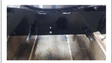
Insert the roller's shafts:
