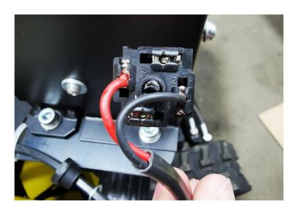
Take off the protection of the side and plug in the alimentation cable.
