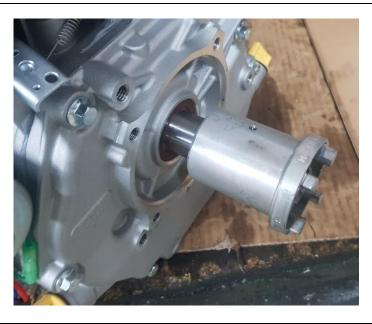
Put the key back on the keypath and install the elastic coupling on the shaft.
