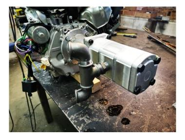
Place the 2 low pressure ¾ elbows on the pump with Teflon.
