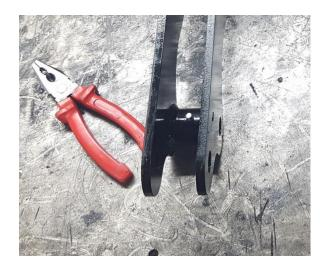
Screw in 2 grease fittings M6 straight on each side of the blade.
