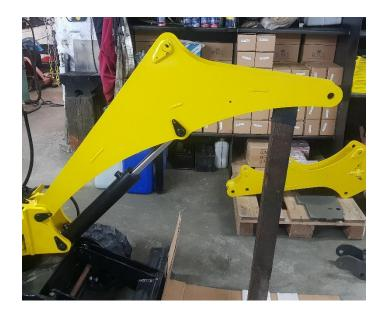
Install the boom and a 30/60 c 300 cylinder with the fitting pointing upward.
