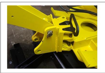
Place the slewing bracket with a  $\emptyset$ 25 lg 210 shaft in the center and a  $\emptyset$ 25 lg 210 shaft with a handle on one of the sides.
