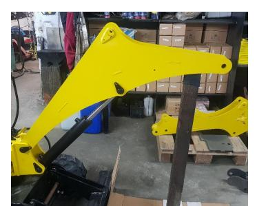
Install the boom and a 30/60 c 300 cylinder with the fitting pointing upward.
