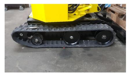
Tension of the tracks : There is no ideal tension, this will depend on the land the excavator has to move on : On a muddy land, the tracks should not be too stretched, it should be a little floppy on the center. On a firm land, the tracks should be stretch almost straight (as on the picture) Do not overtighten the tracks, this will result in premature wear and tear of the tracks and the hydraulic motors.
