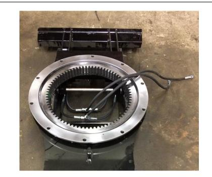
Place the slewing ring on the frame and bolt it down with 16 M12x30 bolts Put threadlocker on each bolt.
