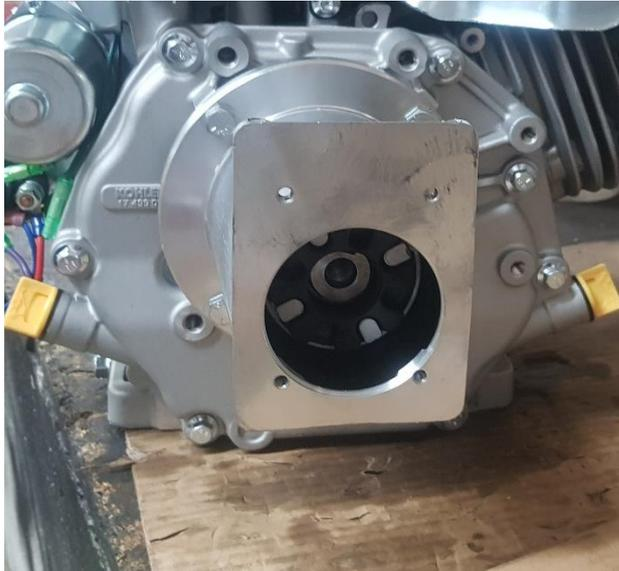
Place the rubber star on the elastic coupling of the motor.
