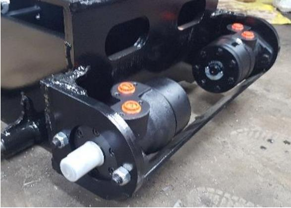
Install 2 hydraulic motors OMR200 on the frame with 2 M12x50 bolts with 2 brake nuts for each motor.
