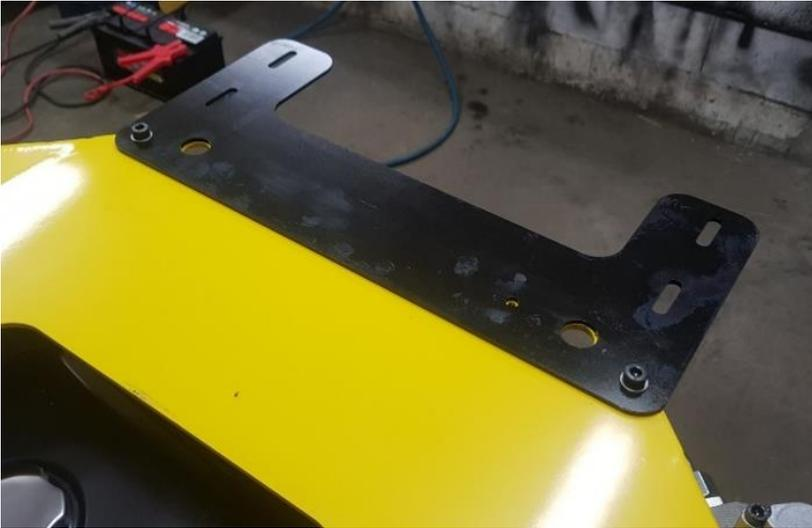
Install the radiator support plate.
