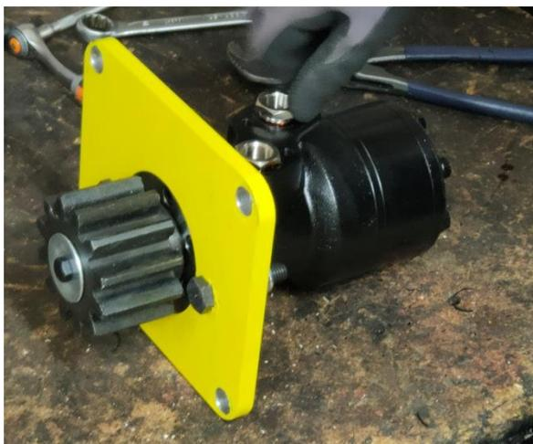
Put with teflon 2 reductions MC1/2-F3/8 on each motor.
