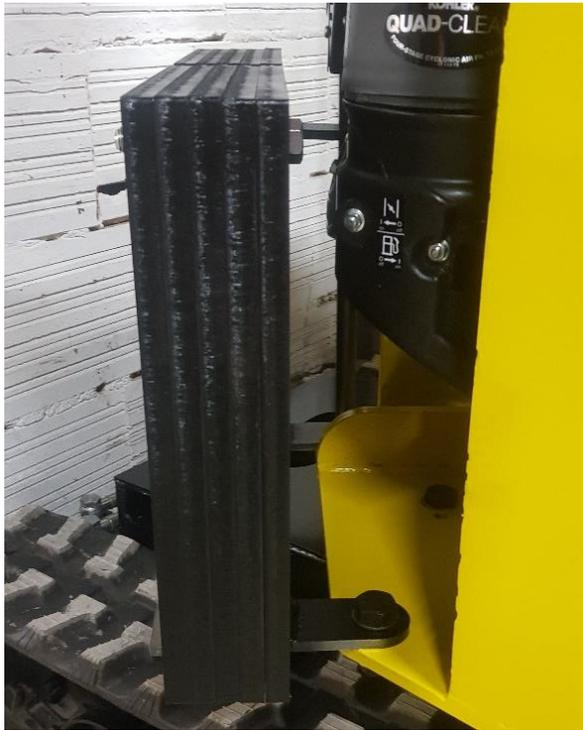
Place the first plate on the pivot axis with a  $\varnothing 20$  lg 430 teardrop shaft and lock it with a 6x16 bolt on the turret.
