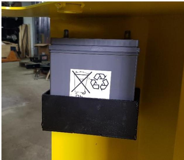
Before installing the engine in the turret, place the battery and support with 2 M8x20 bolts and locknuts.
