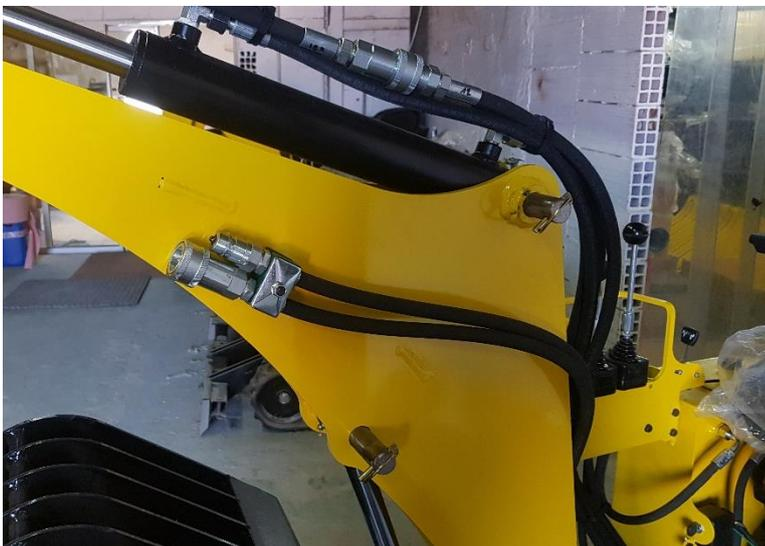
The hydraulic lines for the telescopic arm are 2 hoses connected from the distributor instead of the bypass 15-16 going to the telescopic arm.
