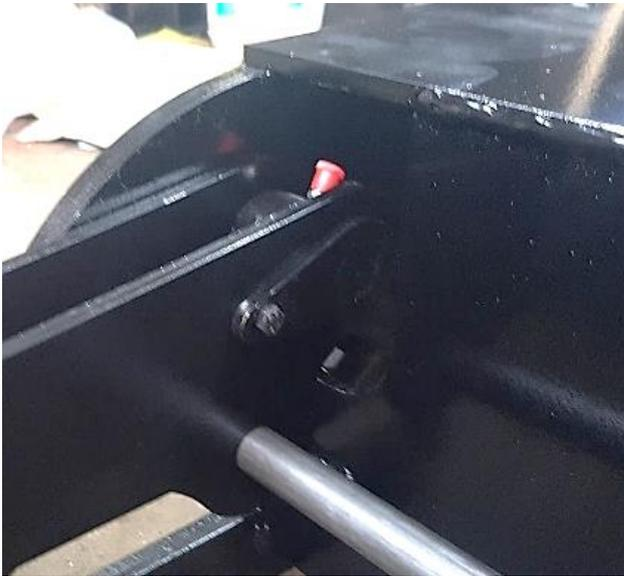
Fix the head of the cylinders with 2  $\varnothing 20$  lg 60 teardrop shaft.
