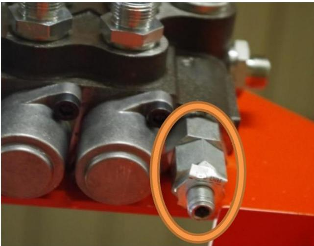
If the excavator lacks power or is under the recommended pressure, you need to adjust the pressure by fist taking off the metal cap on the pressure relive valve then with an allen key screw  $\frac{1}{4}$  turn at a time to raise the pressure or unscrew  $\frac{1}{4}$  at a time to lower the pressure. Do not overtighten as it may cause problems on the hydraulic system.
