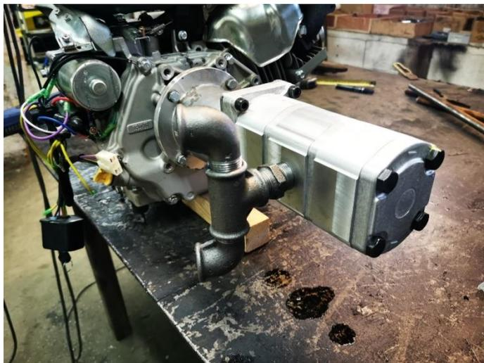
Place the 2 low pressure  $\frac{3}{4}$  elbows on the pump with Teflon.
