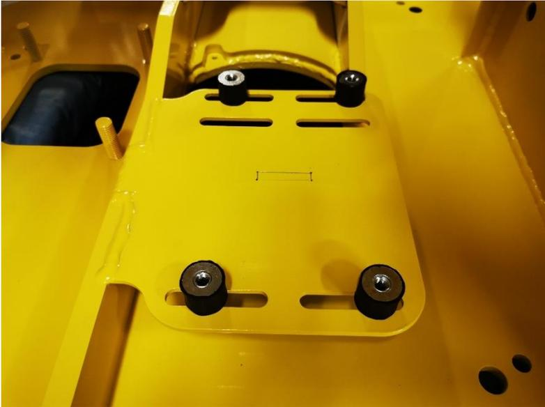
Place the 4 silentblocs with a  $\varnothing 8 \times 30$  washers and a M8 locknut for each; do not tighten them now as it will be easier to install the engine this way.
