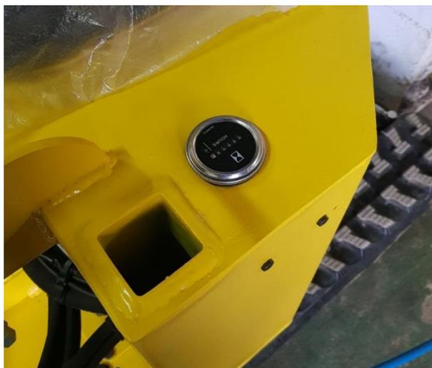
Install the hourmeter in the  $\varnothing 50$  hole on the turret.
