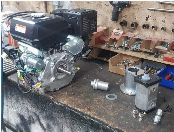
Fill up the oil level, there is 2 plugs on either side of the motor.
