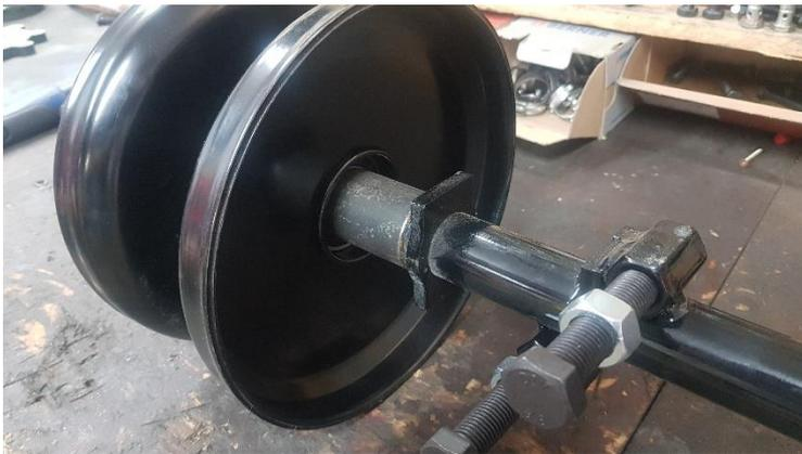
Place the Ø240 – 35 rollers on each side of the axle with a washer between the tube and the roller. Adding some grease facilitate the insertion.
