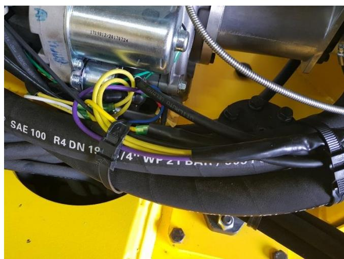
Plug the + terminal of the hourmeter to one of the available yellow wire of the Kohler motor (the 2 yellow wires are + at 12 Volt).
