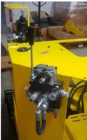
Place the 2 elements distributors at the back of the turret. One joystick spring back in position, put a bypass on this one, the other one stays in place, connect this one according to the guide p 40.
