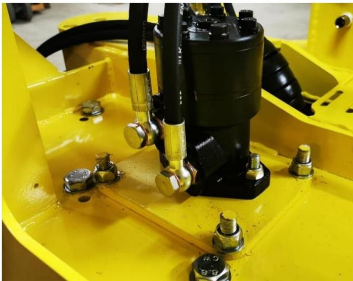
Place the hydraulic motor, be careful that the gears are well aligned.
