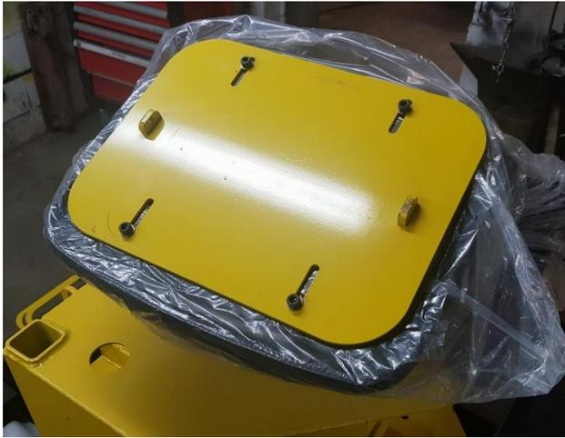
Place the seat on the seat plate, the bolts are mobile, do not hesitate to move them for assembly.
