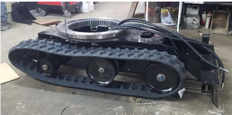
Lift up one side of the frame or the entire frame depending of the equipment available then put on the rubber tracks.
