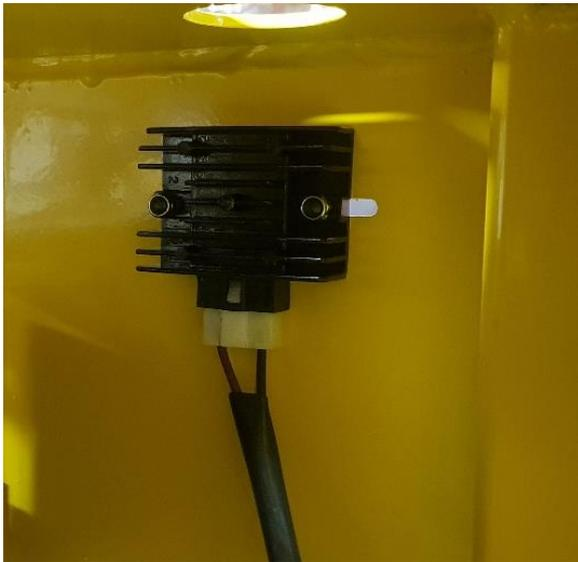
Install the charge regulator to the frame, scrape the paint so that it can have a good connection to the ground.
