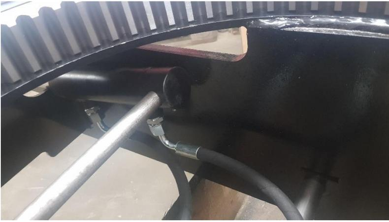
Place the 25x40 c 100 cylinders in the frame with the fittings UM12L pointed downwards and fix the back of the cylinders with a teardrop shaft  $\varnothing 20$  lg 435.
