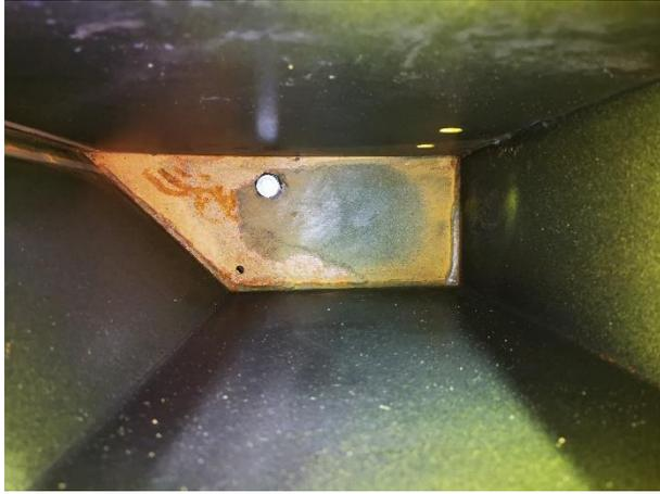
Place a 18x50 bolt with s copper washer and teflon in the tank, lock it tightly in place with a locknut on the other side to avoid any leaks.
