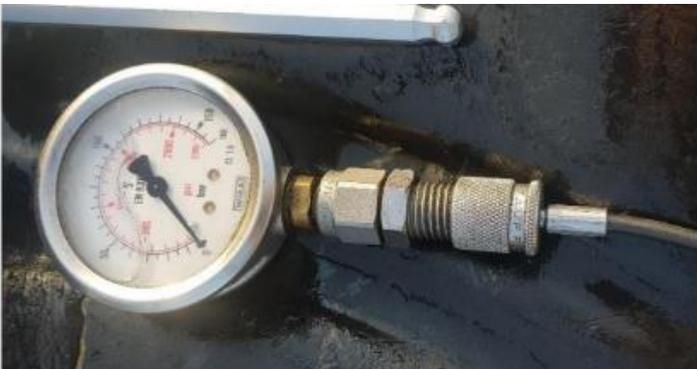
Place the female union  $\frac{1}{4}$  on the manometer and screw the flexible capillary on it.
