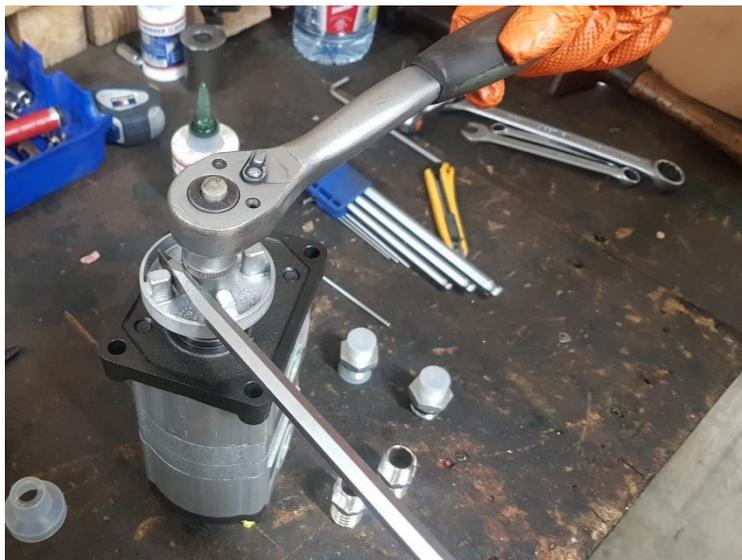
Install the other half of the elastic coupling, making sure that the key does not fall off the keypath of the pump's shaft.
