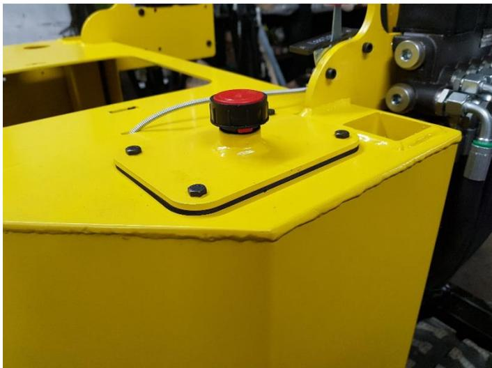
Clean thoroughly the tank and fill it with hydraulic oil and install the tank plate with a rubber gasket and 4 bolts (final level will be done after starting the excavator).
