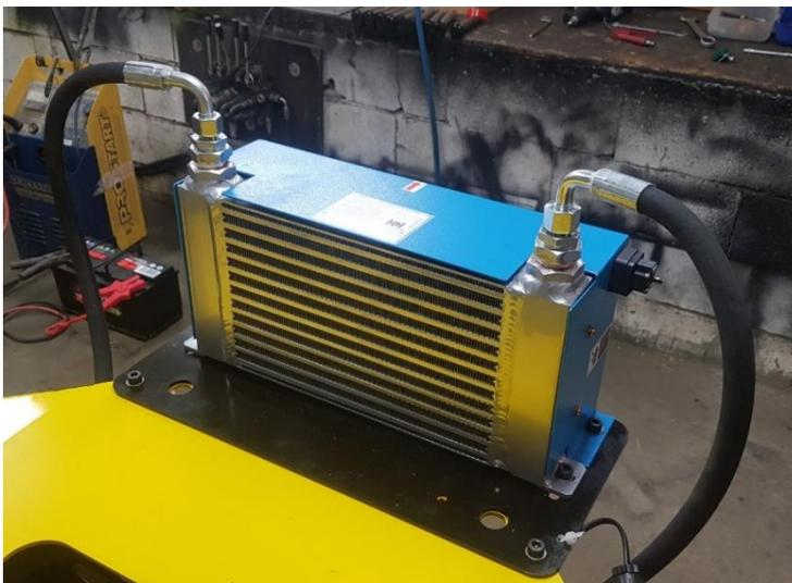
Connect the hoses from the distributor to the radiator then to the tank. See Diagram page 36-37.
