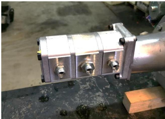
Place 2 fitting UM12L-12x17 on the sides and 1 fitting UM12L-15x21 in the middle.
