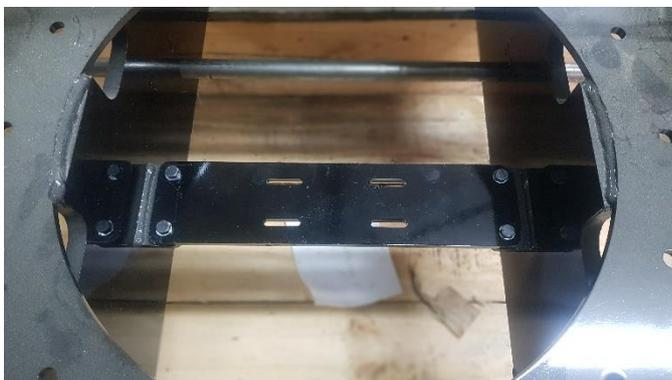
Install the rotary joint support plate at the center of the frame.
