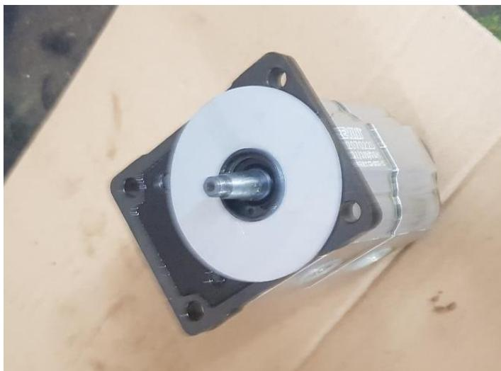
Place the centering washer on the pump.
