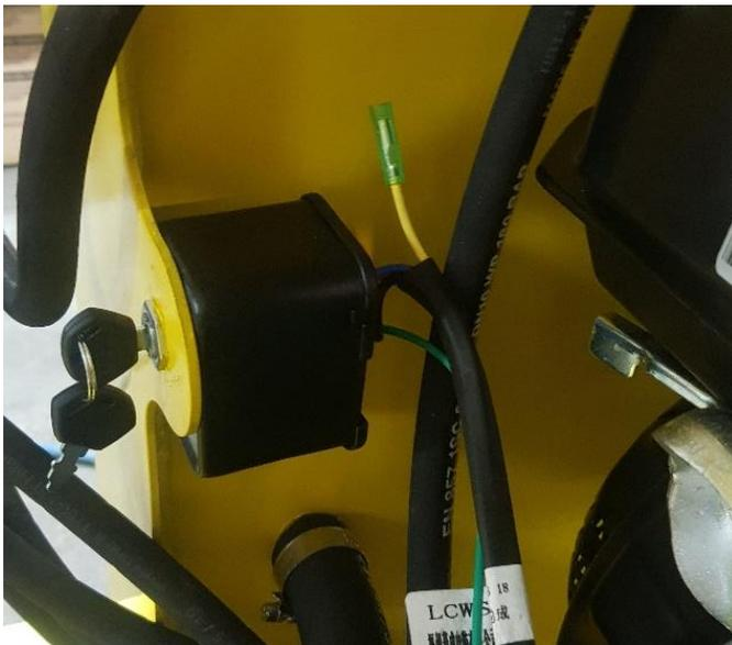
Take the contactor off the motor, cut off the 2 brackets and screw it through the front of the turret.
