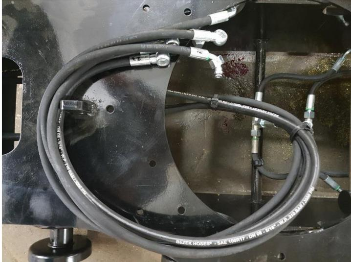
Continue to tie the hoses together with several cable ties so that the ends of the hoses are all about the same level. Using protective sheath is to avoid the hoses being caught in the gear is advised
