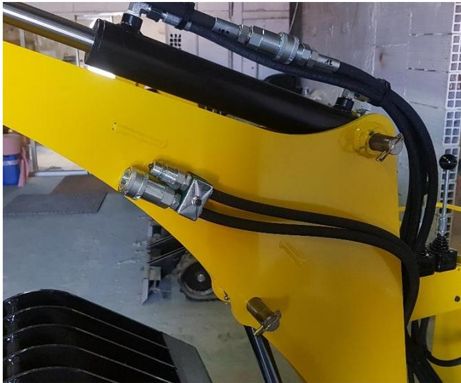
Install the auxiliary hydraulic line from the rear distributor and fix it on the side of the boom.
