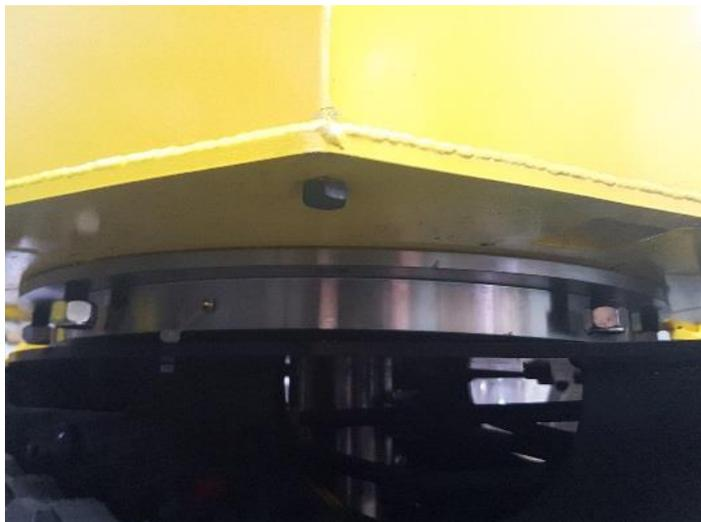
Place the drain bolt M12 x 20 with teflon at the bottom of the tank, screw it tightly in order not to lose oil when filling the tank.
