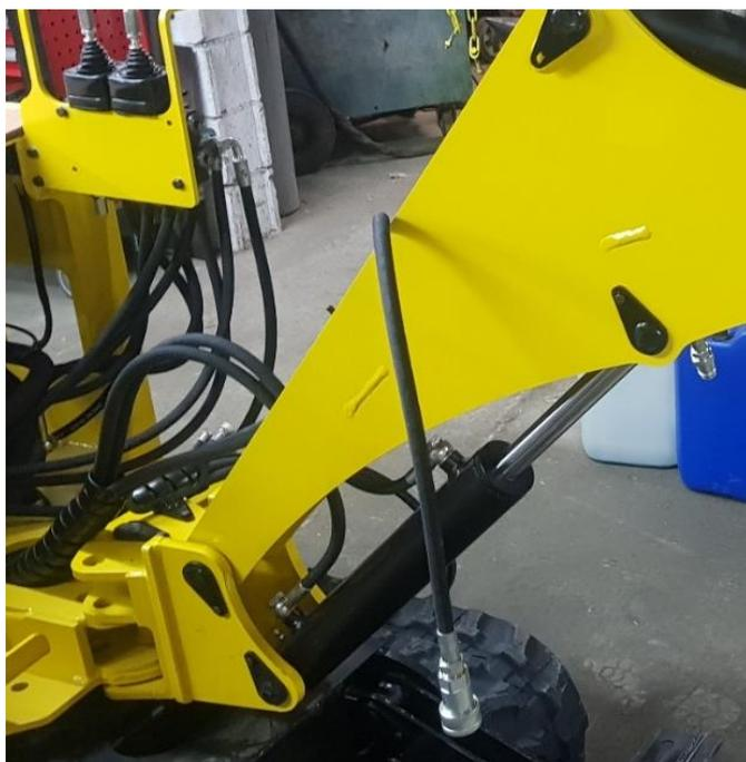
For an easier installation, always connect the hoses starting from the distributor and going to the cylinder/motor.
