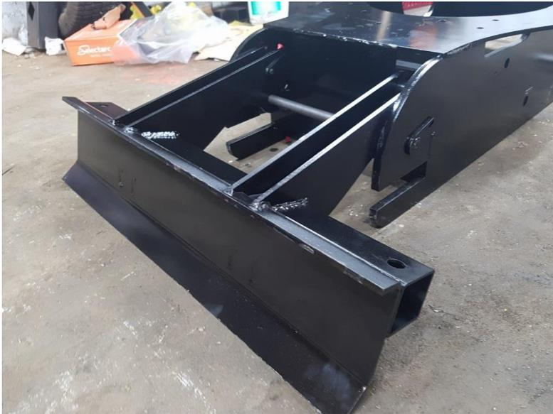
Install the blade with an  $\varnothing 25$  mm length 435 mm teardrop pin from one side to the other of the base frame.
