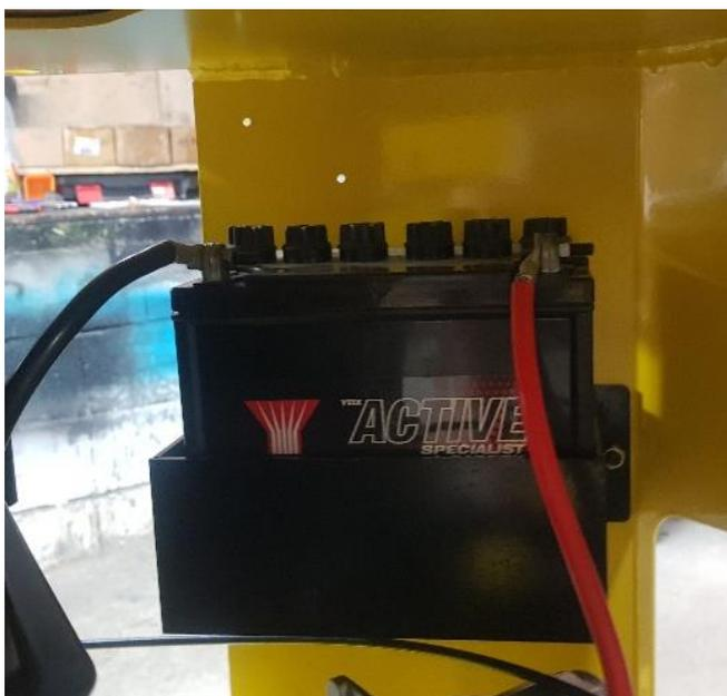
Connect the cable to the battery.
