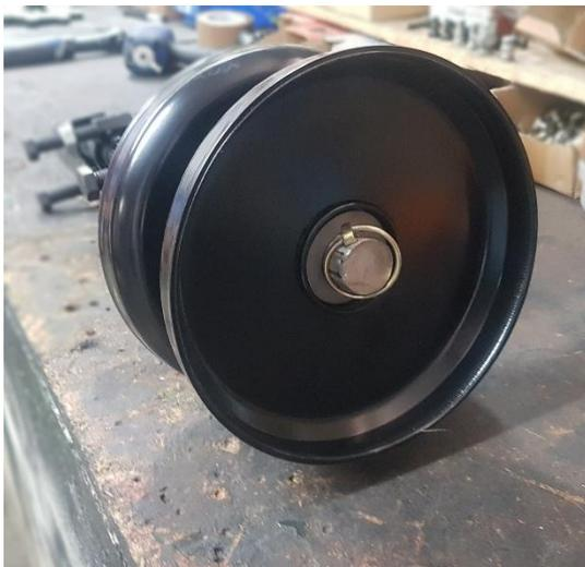
Add 1 pin on each side so that the roller does not slide off the axle.
