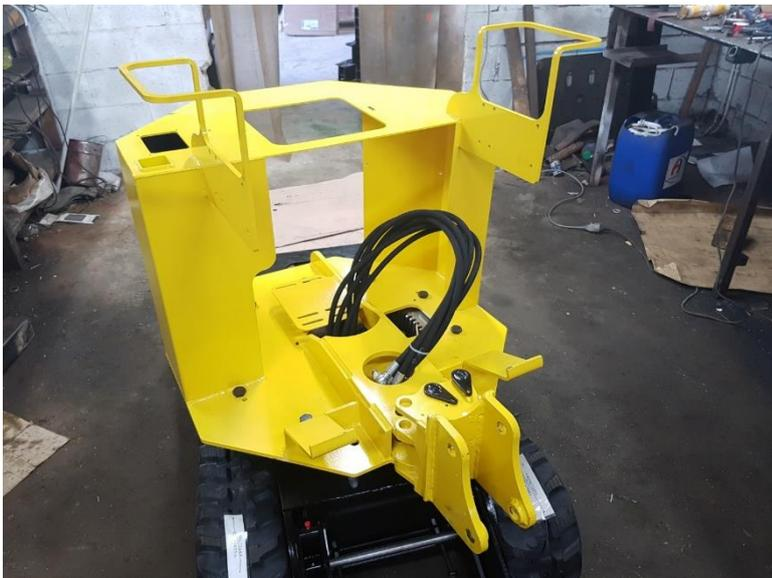
Place the turret on top of the frame while passing the hoses in its center.
