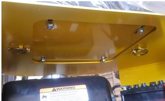
Install the seat on the turret through the mortises and locking it with 2 pins.
