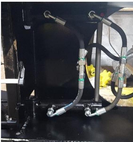
Connect the hoses to the T 12L and the T 12L to the distributor according to the diagram page 42-43.
