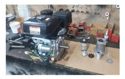
Fill up the oil level, there is 2 plugs on either side of the motor.
