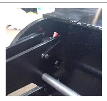
Fix the head of the cylinders with 2  $\emptyset$  20 lg 60 teardrop shaft.
