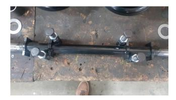
Screw in the 4 16x100 bolts on the front axle with a lock nut on each one.
