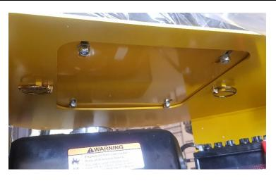
Install the seat on the turret through the mortises and locking it with 2 pins.
