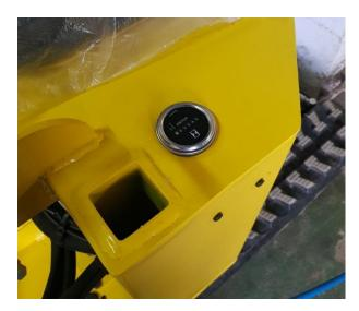
Install the hourmeter in the Ø50 hole on the turret.
