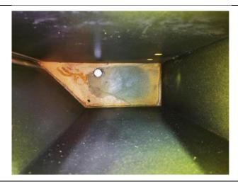
Place a 18x50 bolt with a copper washer and teflon in the tank, lock it tightly in place with a locknut on the other side to avoid any leaks.
