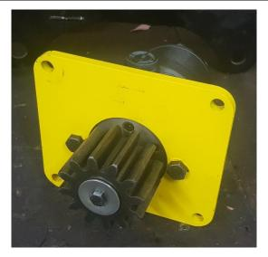
Add the gear to the motor's shaft and lock it in place with a 8x50 bolt + washer and threadlocker.
