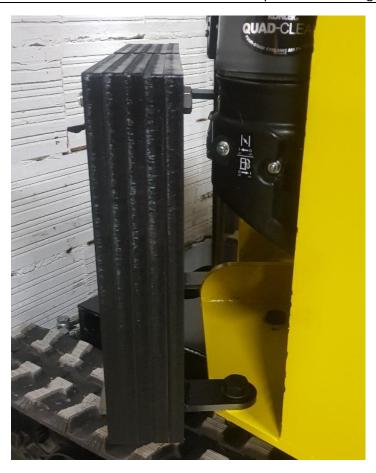
Place the first plate on the pivot axis with a Ø20 lg 430 teardrop shaft and lock it with a 6x16 bolt on the turret.
