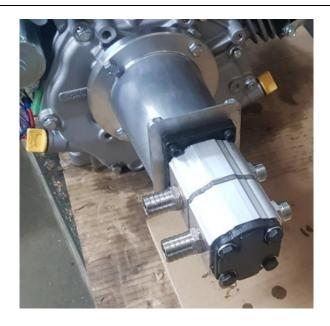
Install the fittings on the pump, 2 UM12L-12x17 on the output, 2 EC19MC3/8 fluted tip on the input with 2 copper washers.
