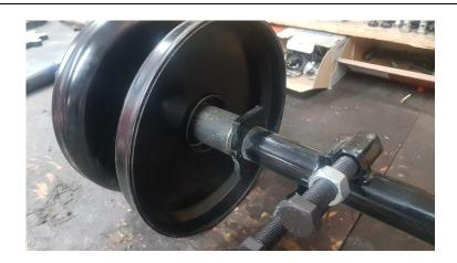
Place the  $\emptyset$ 240 – 35 rollers on each side of the axle with a washer between the tube and the roller. Adding some grease facilitate the insertion.
