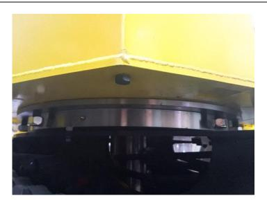
Place the drain bolt M12 x 20 with teflon at the bottom of the tank, screw it tightly in order not to lose oil when filling the tank.
