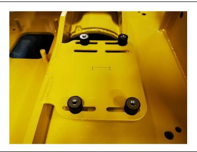
Place the 4 silentblocs with a Ø8x30 washers and a M8 locknut for each; do not tighten them now as it will be easier to install the engine this way.
