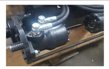
Connect the hoses to the hydraulic motors.
