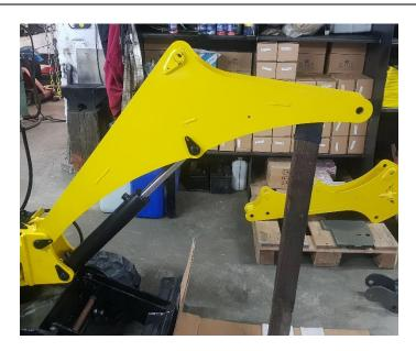
Install the boom and a 30/60 c 300 cylinder with the fitting pointing upward.
