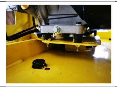
Place the engine on the silenbloc and fix it with 4 bolts M8x35 and washers. Once the 4 bolts are in place, tighten everything.
