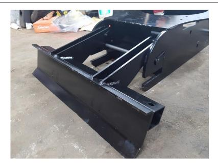
Install the blade with an Ø25 mm lengh 435 mm teardrop shaft from one side to the other of the base frame.
