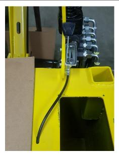
Lubricate the cable with a little oil on each end of the sheath.
