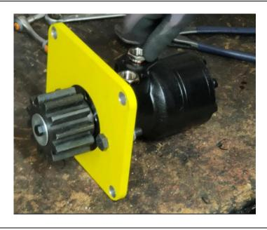
Put with teflon 2 reductions MC1/2-F3/8 on each motor.
