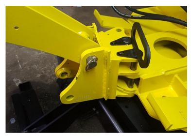
Place the slewing bracket with a Ø25 lg 210 shaft in the center and a Ø25 lg 210 shaft with a handle on one of the sides.
