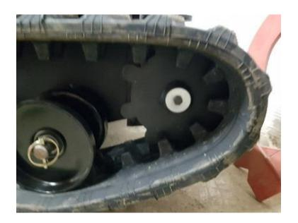
Place the gear in the track and pull it to fit the gear on the motor's shaft, be carefull not to lose the key.
