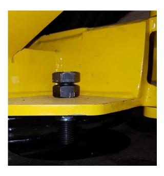
Turn back the turret to its original position and install the stop bolt; it can be placed on either side of the swing bracket.
