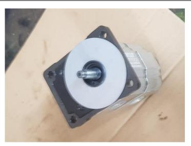
Place the centering washer on the pump.
