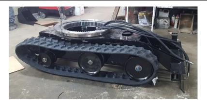
Lift up one side of the frame or the entire frame depending of the equipment available then put on the rubber tracks.
