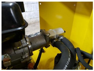
Connect the input of the pump to the tank and the output to the distributors (see p35).
