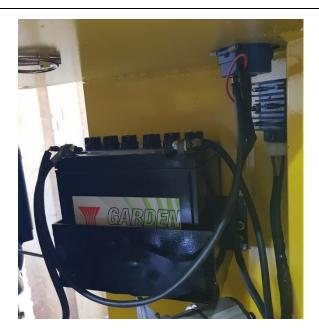
Plug the – terminals of the hourmeter to the terminal – of the battery.
