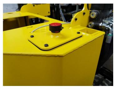
Clean thoroughly the tank and fill it with hydraulic oil and install the tank plate with a rubber gasket and 4 bolts (final level will be done after starting the excavator).
