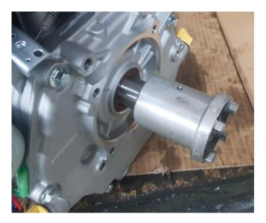
Put the key back on the keypath and install the elastic coupling on the shaft.
