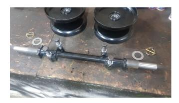
Insert a Ø42 lg 55 tube on each side of the front axle to space the rollers.
