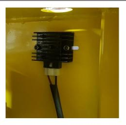
Install the charge regulator to the frame, scrape the paint so that it can have a good connection to the ground.
