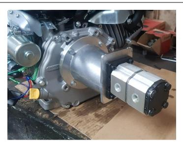
Place the pump on the lantern with 4 BTR 6x25 bolts and threadlocker.
