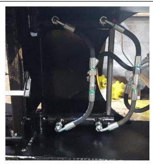
Connect the hoses to the T 12L and the T 12L to the distributor according to the diagram page 37.
