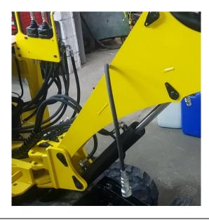
For an easier installation, always connect the hoses starting from the distributor and going to the cylinder/motor.
