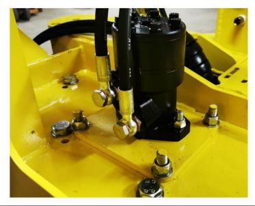
Place the hydraulic motor, be careful that the gears are well aligned.
