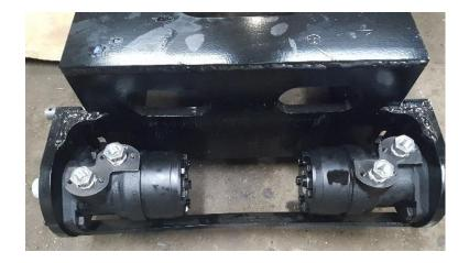
Put with teflon 2 reductions MC1/2-F3/8 on each motor.
