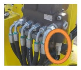
Begin by looking for the pressure relieve valve, this will indicate the entry side of the hydraulic oil and will allow the adjustment of the pressure.
