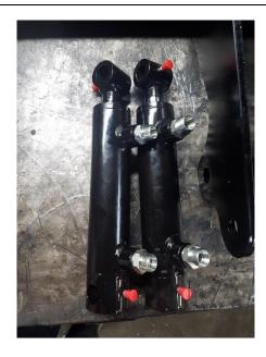
Screw in the 4 fittings UM12L-12x17 on the cylinders VD25x40 c 100.
