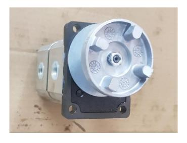
Install the other half of the elastic coupling, making sure that the key does not fall off the keypath of the pump's shaft.
