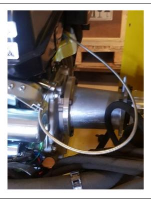
Pass the cable through the guide, making a loop wide enough so that the cable does not have too much resistance while being used.
