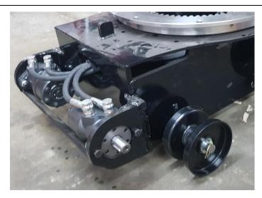
Before installing the rubber track, place the gear on the hydraulic motor and adjust if if need be.
