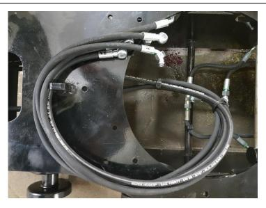
Continue to tie the hoses together with several cable ties so that the ends of the hoses are all about the same level.
