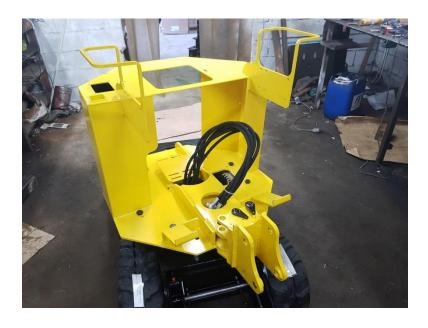
Place the turret on top of the frame while passing the hoses in its center.
