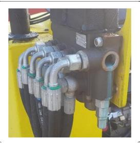
Put all the component of the excavator on the ground and move the 2 controllers on every direction to relive the pressure of the system.
