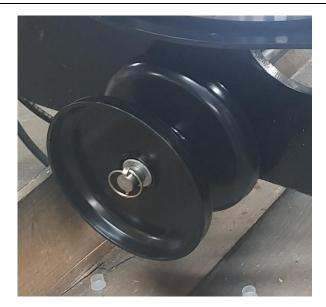
Place 2 Ø25 washer on each side of the roller before placing the pin.
