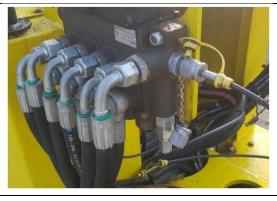
Screw the capillary on the union placed on the distributor.
