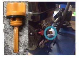
The motor oil level can be checked from ether sides by unscrewing the gauge and controlling the level on the graduation.
